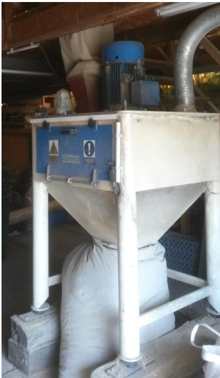
Figure 8 Hammer mill ŠV- 15
