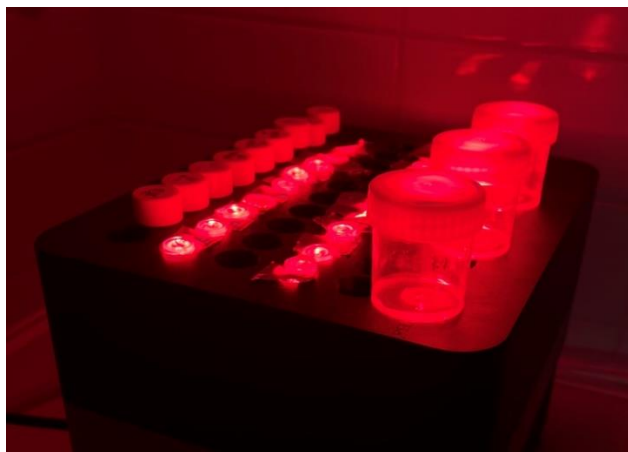
Figure 14 The illumination of the samples inside the holder on the LED array.
