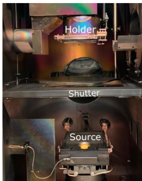
Figure 9 Photo of components inside the E-beam evaporator chamber.
