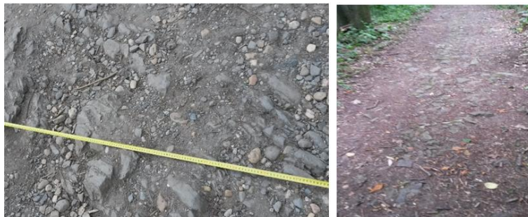
Figure 23 - Example of coarse-textured and low organic matter with low soil moisture on trail tread that would probably reduce soil erosion that could result to incision. (Photograph by Phaniel Gade)
