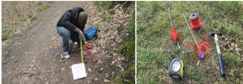
Figure 6 - An illustration of how maximum incision was recorded using a nylon string fastened between two metal pegs that can describe the tread boundaries (Photographs: Gade, 2015)
