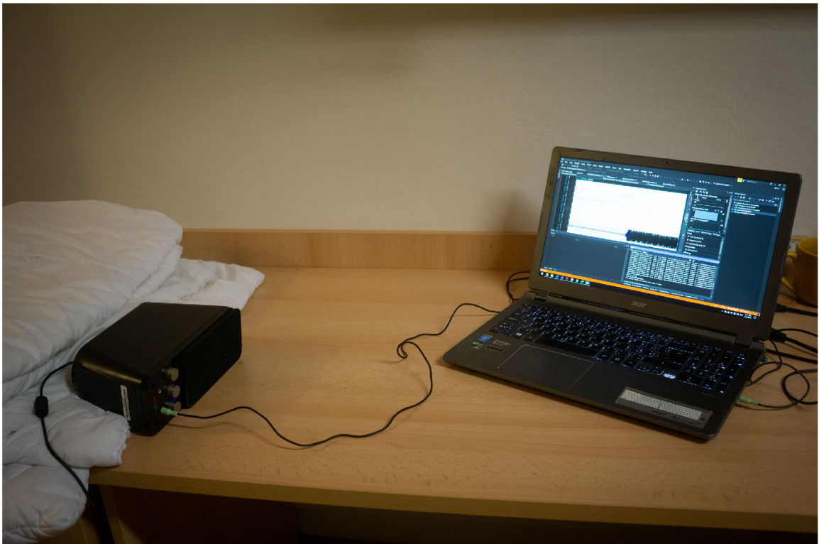
Figure 5.14: One of the testing configurations. Similar one was used in generating Figure 5.8 . Mono speaker connected to a laptop with integrated mic. The speaker is laid down to enable better directing of sound waves.
