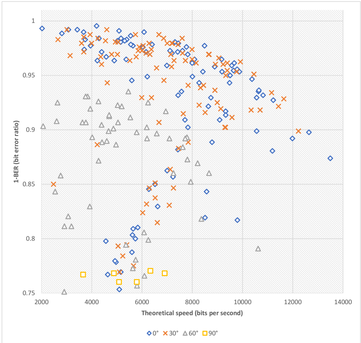
Figure 5.9: Test with different angles of the speaker facing the microphone. Distance between devices was 75 cm. 0° is the speaker directly facing the microphone.
