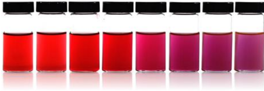
Figure 4: Solutions of various sized monodispersed gold nanoparticles. Size of nanoparticles in solutions is increasing from the left (red color) to the right (purple color) [26]
