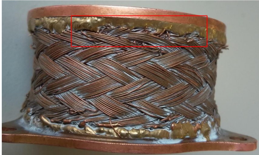
Picture 4.1 CTB with marked welds and free wires
