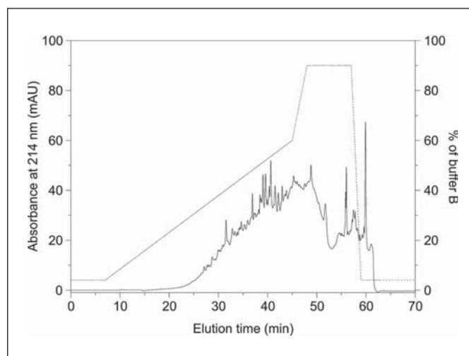
**Fig. 3.** Gradient reversed-phase nanoflow chromatographic separation of tryptic peptides produced by in-gel digestion with trypsin. The samples were separated by nanoLC. The chromatogram shown was generated from slice No. 6 in figure 2. The solid line represents absorption at 214 nm, the dotted line refers to the gradient of mobile phase B.
