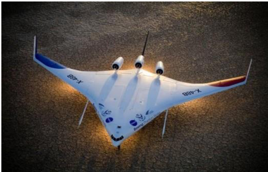
X-48B aircraft, Blended Wing Body concept. (Source: profimedia.cz)
