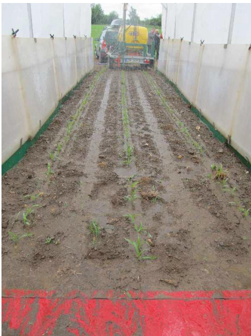
Apx Figure 4: Rainfall simulation on the plot with vertical tillage practice (VUMOP, 2015).
