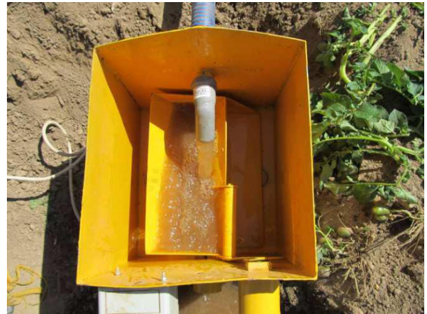
Apx Figure 3: "Flip" device - RS is equipped by the flipping device which measure the SR by numbers of flips (VUMOP, 2015).
