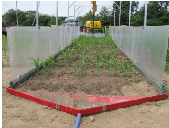
Apx Figure 6: Simulator - capturing the runoff of rainfed surface.
