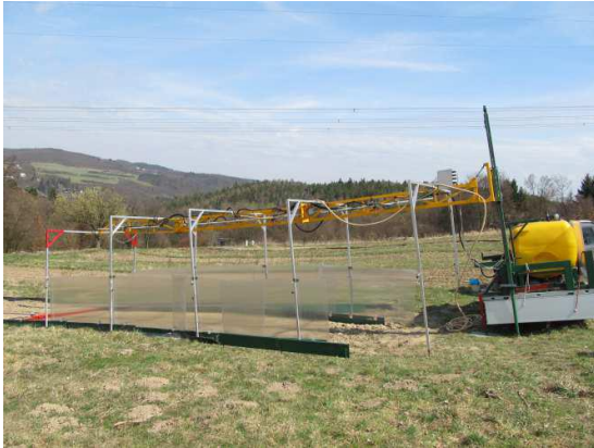
Apx Figure 2: Rainfall simulator opened up on site (VUMOP, 2015).
