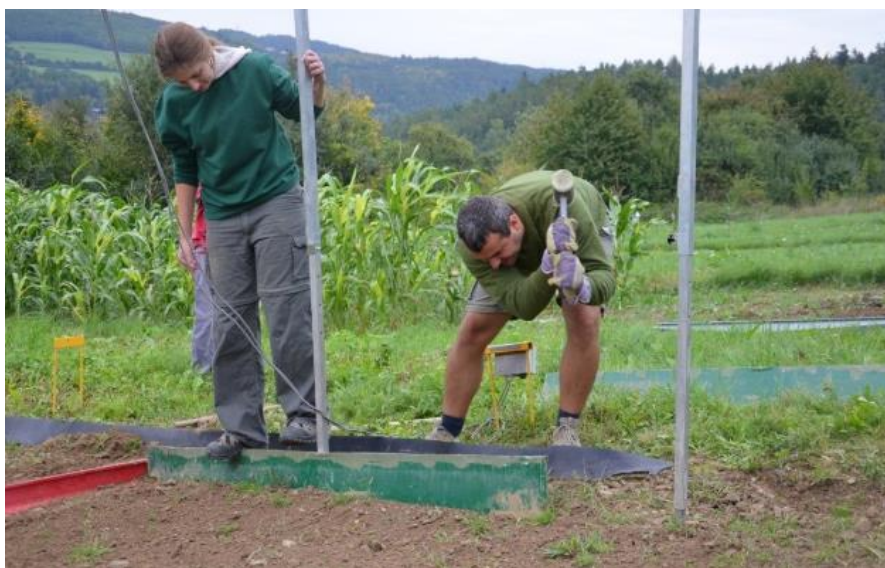
Apx Figure 1: Setting up the simulator on site (VUMOP, 2015).
