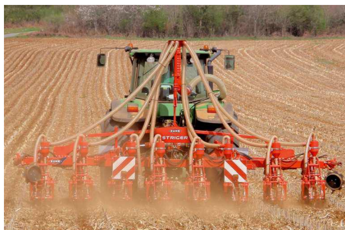
Apx Figure 8: Strip tillage with machine KUHN-STRIGER (VUMOP, 2015)
