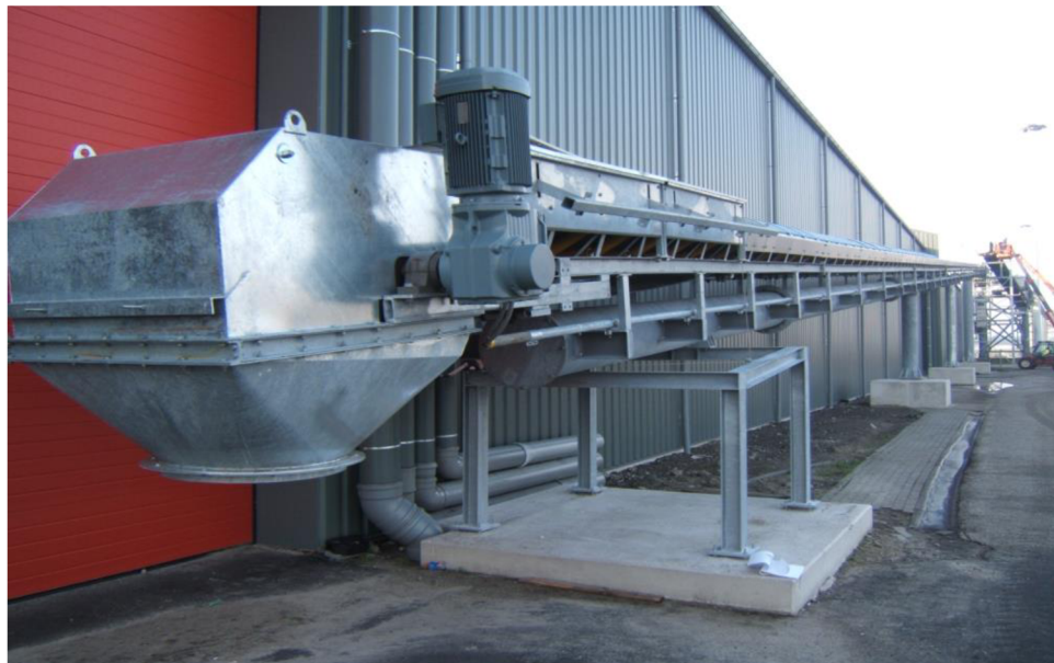
Fig. 3.3: Heavy-Duty Belt Conveyor (Jansen & Heuning www.jh.nl , 2023)
