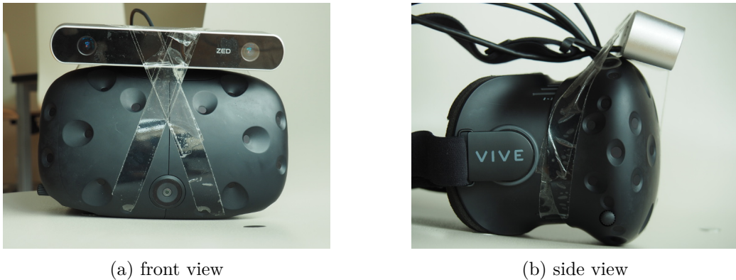
Figure 4.2: The ZED camera attached to the HTC Vive HMD. Figure 4.2a shows both from the front. Figure 4.2b better shows the position and rotation of the ZED relative to the HMD.
