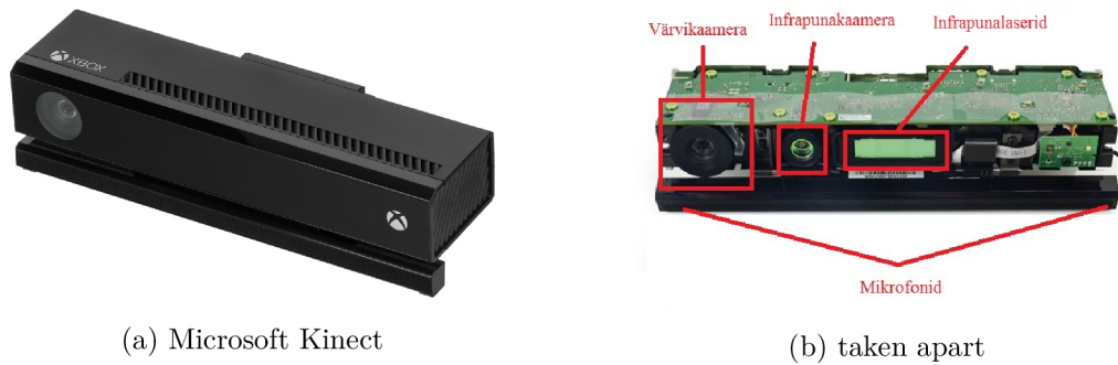
Figure 2.2: Photos of Kinect for Xbox One. Figure 2.2a shows the whole device with only the color camera visible (source:[4]). In figure 2.2b (source: [15])the color camera is in the leftmost red square. The rectangular part in the middle is the IR emitter and between the aforementioned two is the IR sensor.
