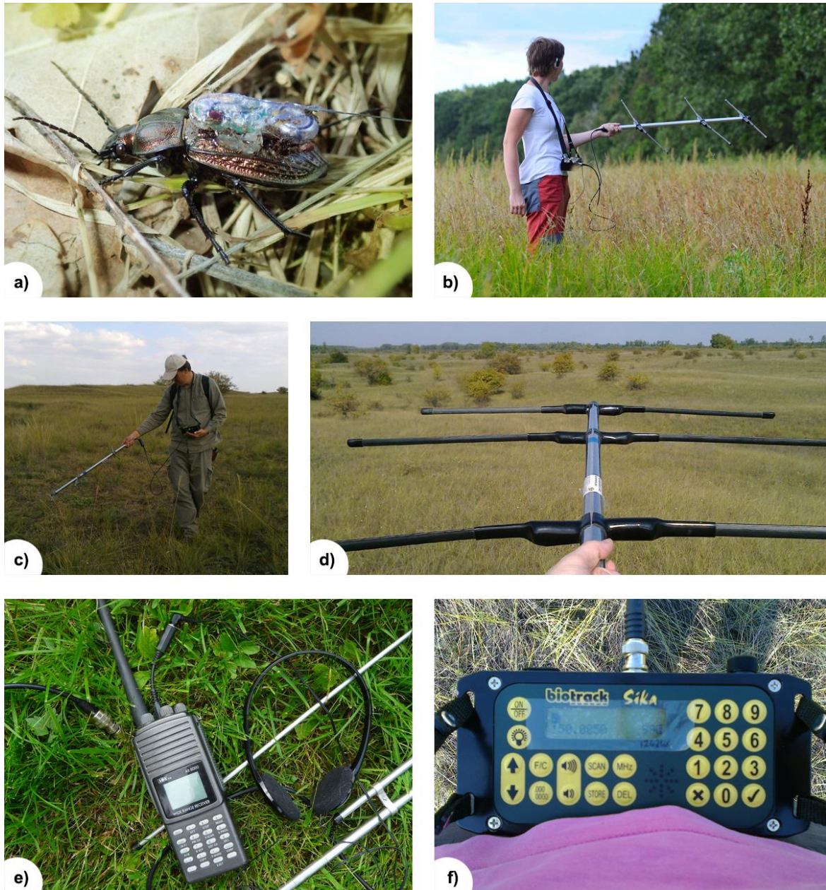
Figure 2: Principal components of radio telemetry. An active transmitter (tag) attached to a ground beetle by glue (a) consists of a transmitting unit, an emitting antenna and a power source, i.e. battery. Tag emits regular pulses of fixed very high frequency, usually in MHz, which is unique for each tag. The signal of the tag is detected by hand-held receiving antenna system, such as multiple parallel elements compiled in a line (Yagi, b, d) or a short dipole antenna (e), and processed by a receiver (e, f). During tracking, the tracking person sets the tag frequency into receiver and sweeps the receiving antenna from side-to-side to determine the direction of the strongest signal (b, c).
