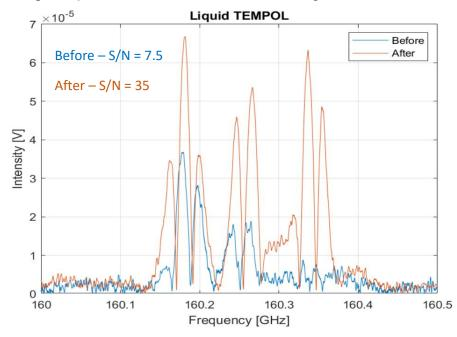
Fig. 8.1 Recorded spectra of the liquid TEMPOL before and after applying the automated coupling with values of signal to noise (S/N) ratios
