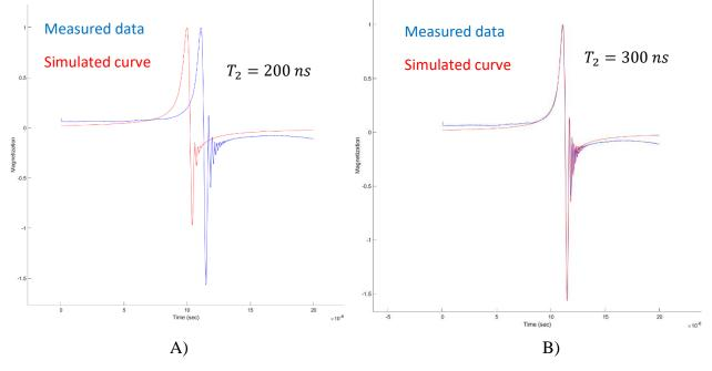
Fig. 8-3 A) Wrong fitting, too low relaxation time. B) Precisefit of parameters of the measurement with resulting relaxation time  $T_2 = 300 ns$
