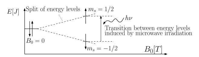
Fig. 2-2 Linear splitting of spectral lines and the increasing energy difference between states in the increasing outer magnetic field  $B_0$  [8]
