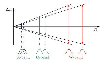
Fig. 3-1 Two species of different g-values are very difficult to distinguish at the X-band frequency. The situation is better for Q-band, but the lines are fully separated only for W-band [2].
