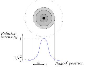
Fig 4-4 Intensity distribution of the Gaussian beam in the mode 0;0. The image was taken and adjusted from [17].
