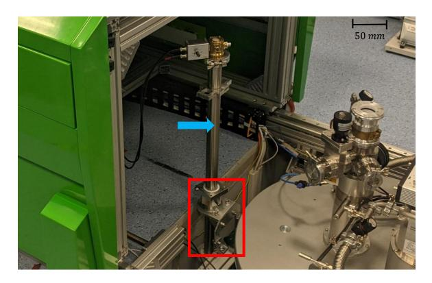
Fig. 6-2 Attached testing holder to the framework (red rectangle) with inserted probe (blue arrow)
