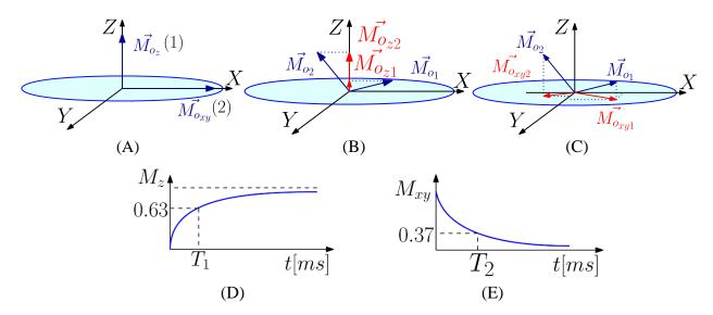
Fig. 2-3 A) System shortly before irradiation, the maximal amplitude of  $M_o$  in z-axis (1), Immediately after irradiation, maximal projection of  $M_o$  in x-y plane (2). B) Z-vector of  $M_o$  regaining its strength. C) Vanishing x-y projection of  $M_o$ . D)  $T_1$  relaxation E)  $T_2$  decay
