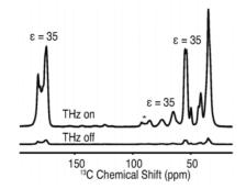
Fig. 2-4 Significantly enhanced signal after application of DNP method and 0.263 THz radiation on the samples of amyloid fibrils by [38]. The figure is taken from [38] and adjusted.
