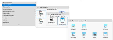
Fig. 7-2 Library for manipulation with data from Lock-in amplifier by Zurich Instruments
