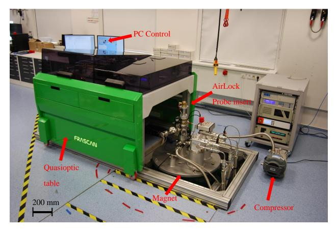
Fig. 3-3 Frequency Rapid Scan Electron Spin Resonance spectroscope (FRASCAN) Actual spectroscope set up as of March 26 2021
