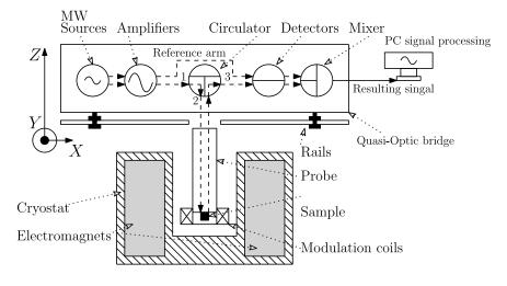
Fig. 3-4 Scheme of the spectroscope hardware with the mw radiation path
