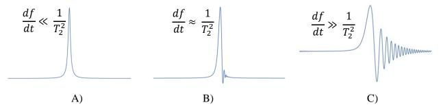
Fig. 3-3 A) Condition for the rapid scan was not met and the recorded spectrum is classical frequency domain sweep. B) The speed of a frequency sweep rises but still is not enough. C) Condition for the rapid scan method is met and the frequency sweep is considerably larger than the relaxation time hence the rapid scan spectrum may be recorded and observed. Pictures taken and adjusted from [47]
