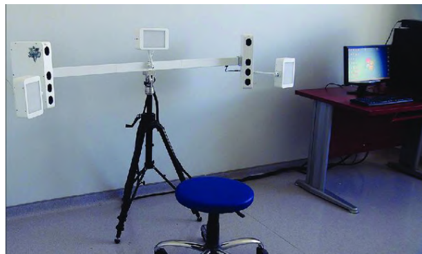
Figure 1.2: Illustration of photogrammetry principle on the left [30], photo of a stereophotogrammetry camera setup [23] on the right.
