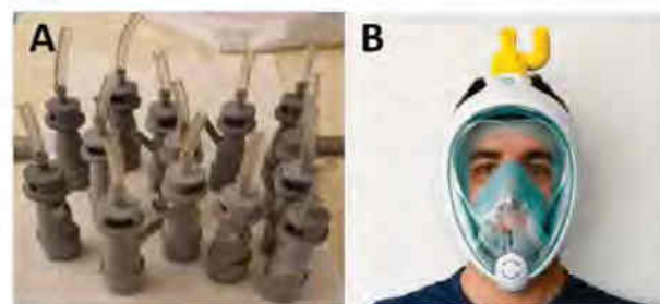
Figure 4. A) 3D-printed venturi respirator valves by Italian company. Reproduced with permission [106] Copyright 2020, ISINNOVA S.R.L. B) Snorkeling EasyBreath masks connected to Charlotte Valves. Reproduced with permission. [107] Copyright 2020, ISINNOVA S.R.L.
