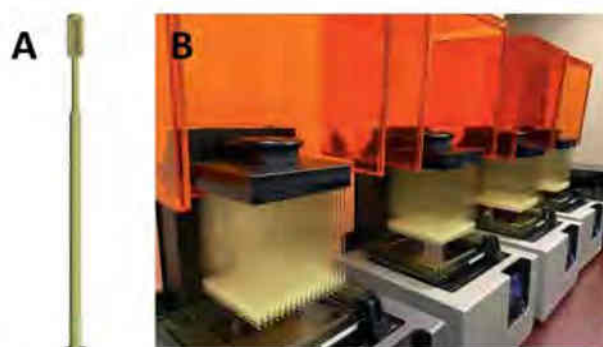
Figure 5. A) NP swabs designed using computer-assisted drawing (CAD) software. B) 3D-printed NP swabs produced in bulk, ready for post-processing. Reproduced with permission under the terms of the Creative Commons CC BY 4.0 license. [115] Copyright 2020, the Authors. Published by Springer Nature.
