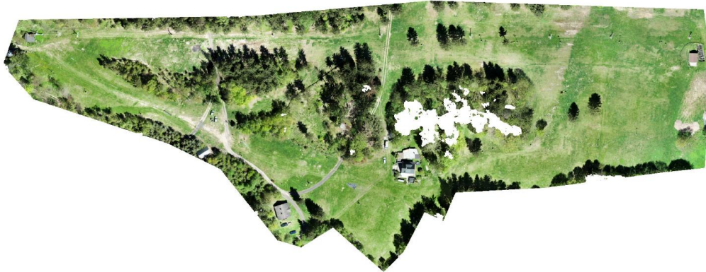
Fig. 7-d: Alšovka ski resort. Images were taken for the purpose of creating orthophotos and DEM was created by M.Součková. The white places signify DEM holes – the flight was not preplanned to fly over the forests. Coordinate system: S-JTSK / Krovak East North (EPSG::5514).
