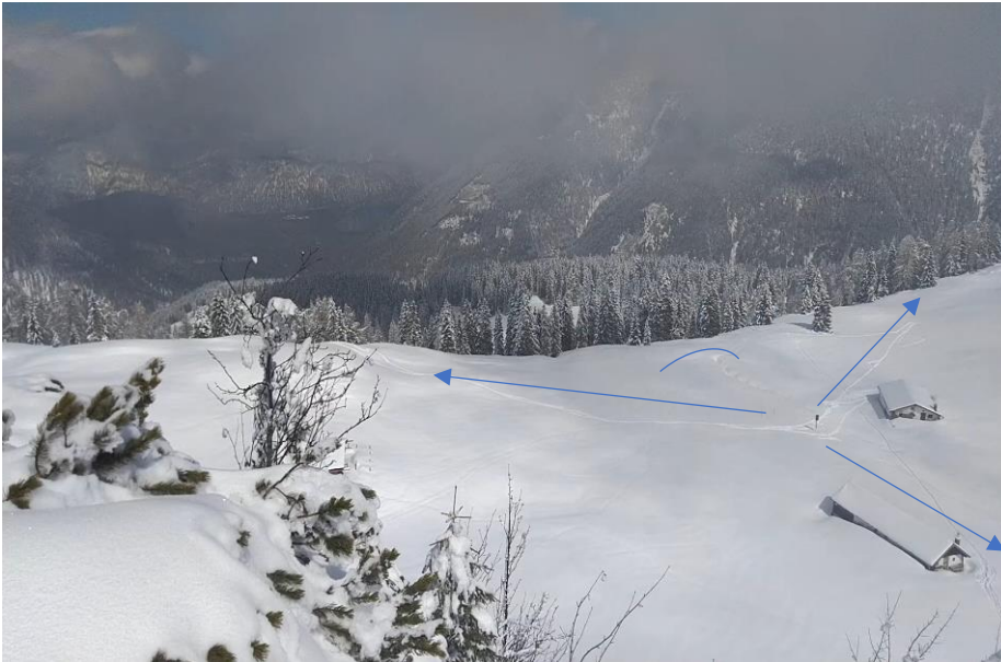
Fig. 8-k: In situ SD and SWE collection methodology: three lines under 120 ° at Lechkogel station.
