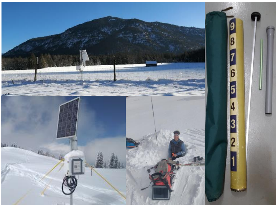
Fig. 8-j: Cosmic-Ray Gauge in Graswang (upper left), and in Lechkogel (lower left) and Snow tube (right).
