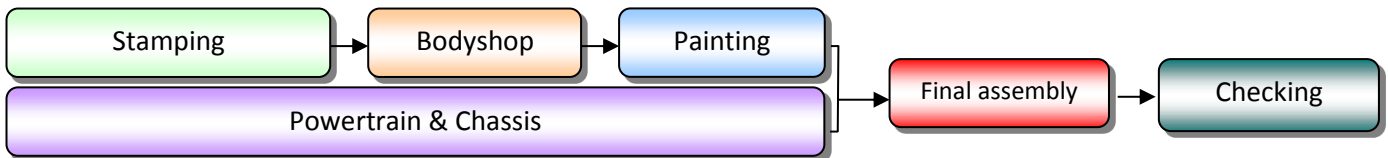
Figure 5 Plant flow synoptic
