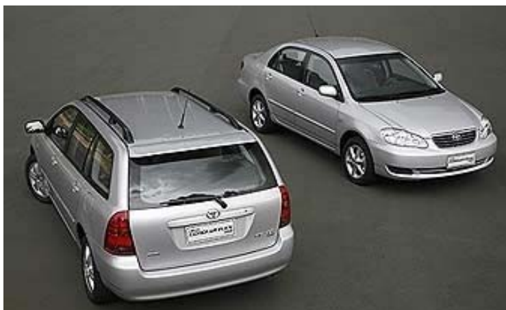
Obr.12 : Toyota Corolla XLi a Fielder, oba se systémem flex-fuel; 1,8l; 136hp
