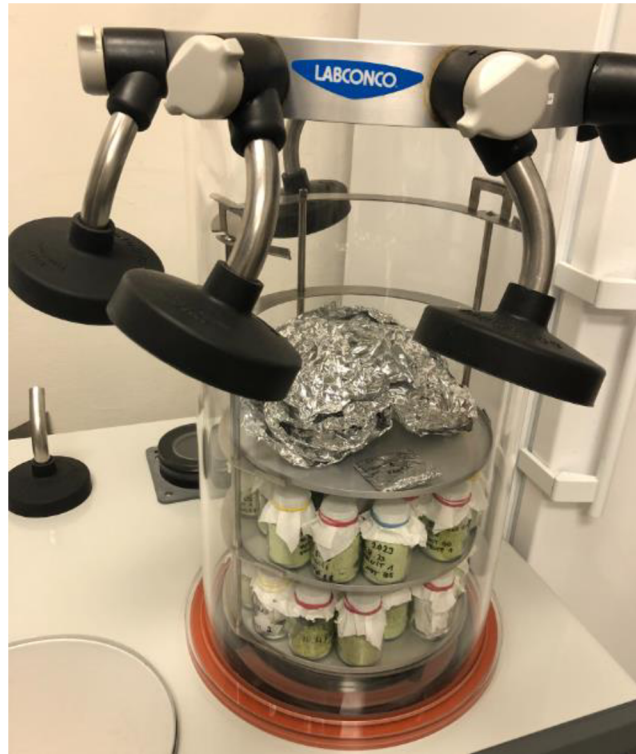
Figure 9: Lyophilization of zucchini samples (own photo documentation).
