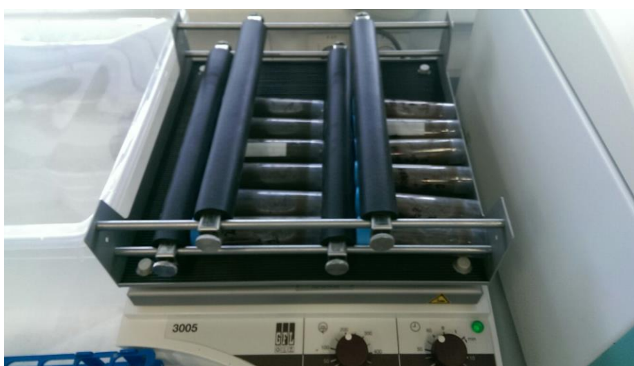
Figure 6. Horizontal shaker (GFL 3005, Germany) for continuous mixing of soil and water.
