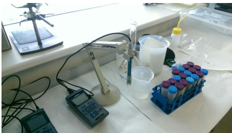
Figure 7. Measurement of pH, Eh and EC of the soil samples.
