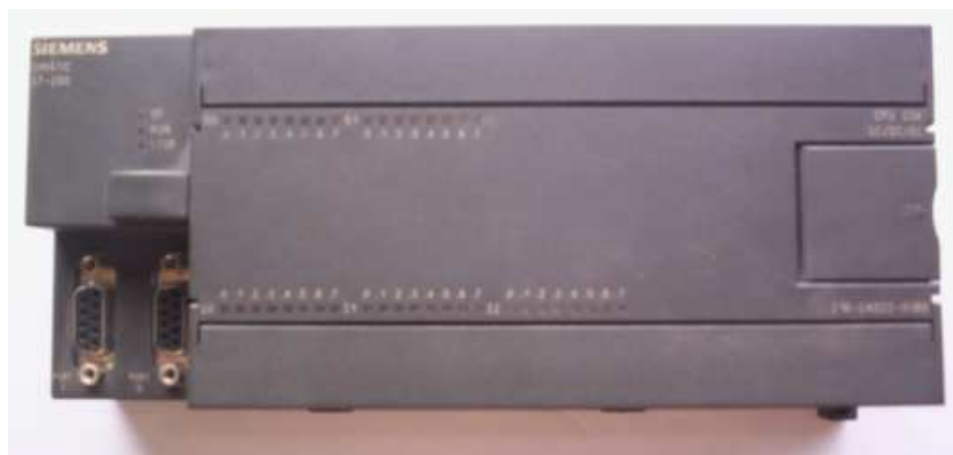
Obr. 3.1 PLC Simatic S7-200 s CPU 226
