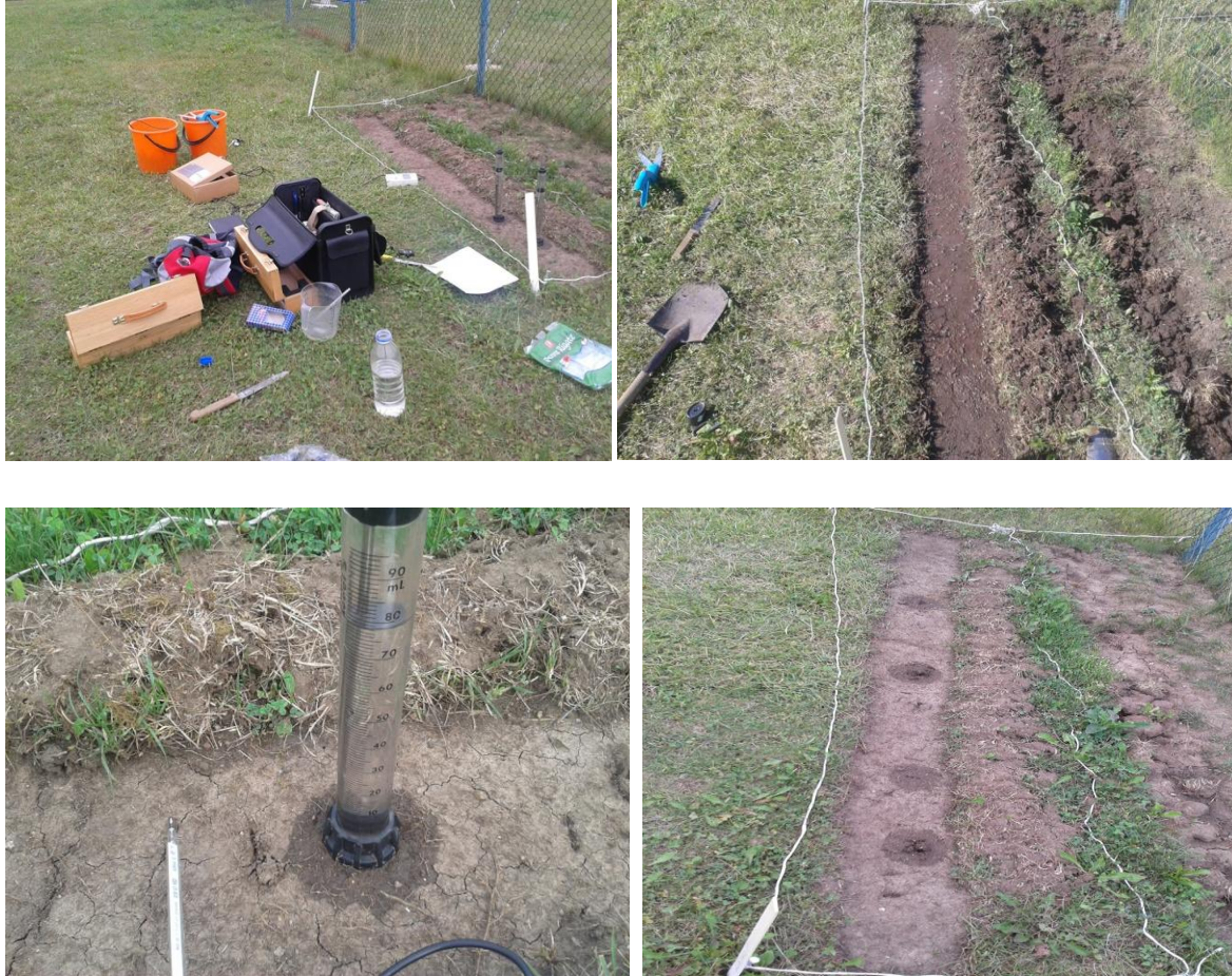
Fig.4.4 Pictures taken during field measurement of unsaturated hydraulic conductivity (June, 2013)
