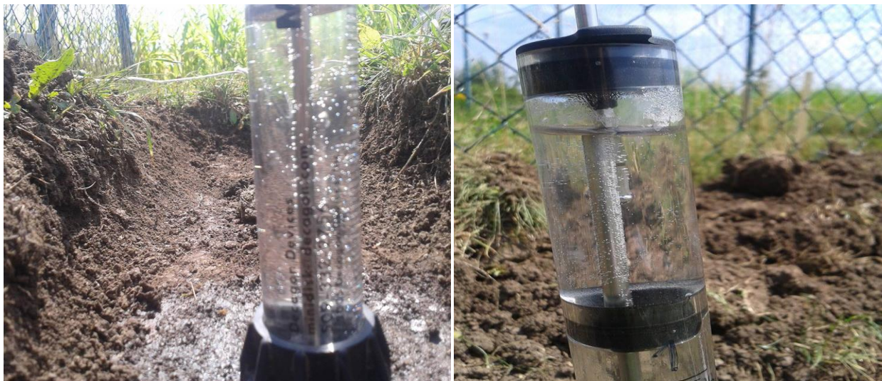
Pictures that show air bubble formed at field measurement in summer in minidisk infiltrator reservoir and bubble chamber respectively
