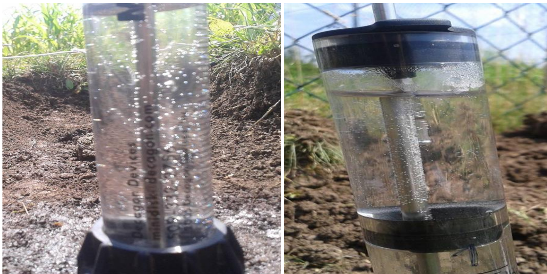
Fig.5.4 Pictures taken to show air bubble formed during field measurement due to surrounding high temperature
