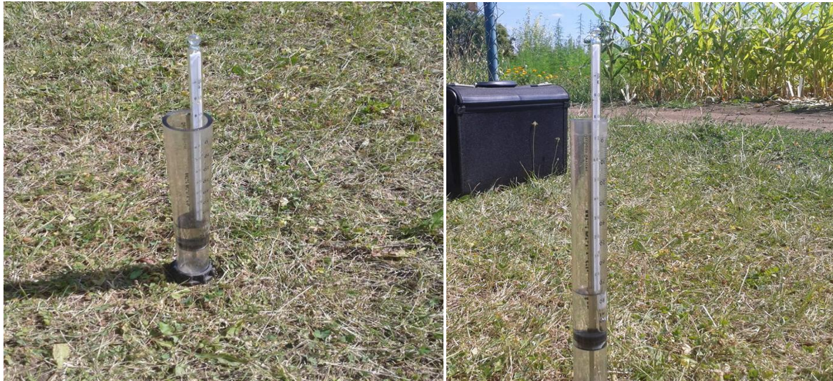
Pictures taken during water temperature measurement in minidisk infiltrator reservoir after infiltration measurement using thermometer
