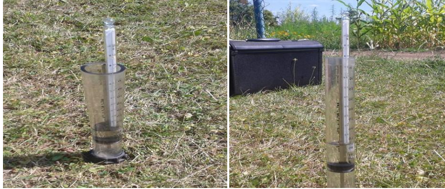
Fig.5.5 Pictures taken which show water temperature measurement in MDI reservoir after final infiltration at field
