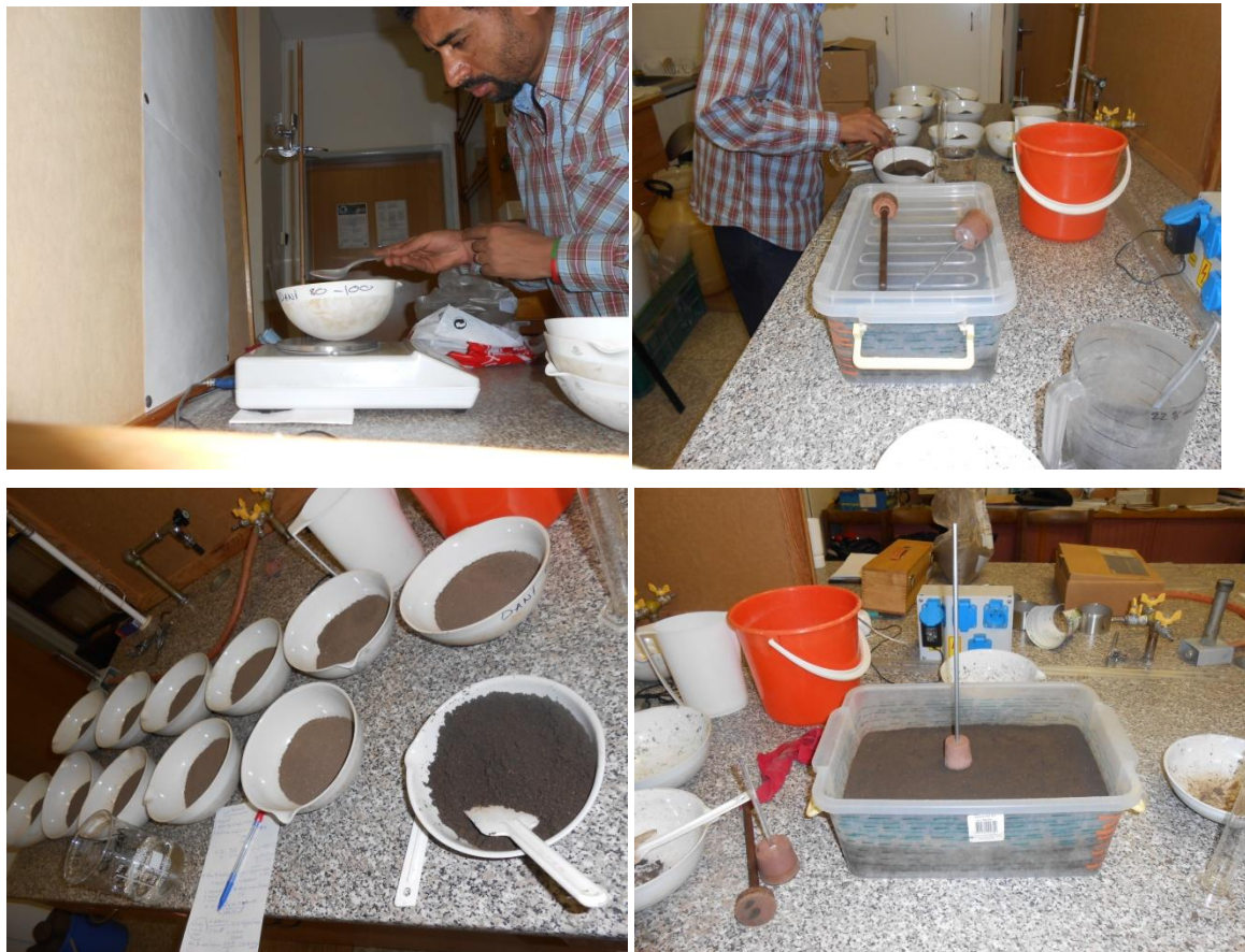
Fig.4.5 Pictures taken in laboratory weighted soils, soil with 20% water content by volume and compacted soil.
