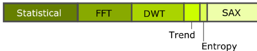
Figure 24: Time-lapse feature extraction from the univariate time series. Extracted time-lapse features are assembled into a partial time-lapse feature vector. Individual segments represent the group of time-lapse features obtained by the particular extraction technique. The length of the segments indicates the approximate number of extracted time-lapse features for the particular group.
