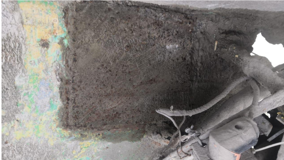
Figure 10: Patchwork in mother plate [20]
