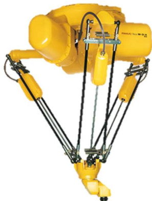
Obr. 3.4 – Delta robot Fanuc M-3iA/6A, dostupné z [33]
