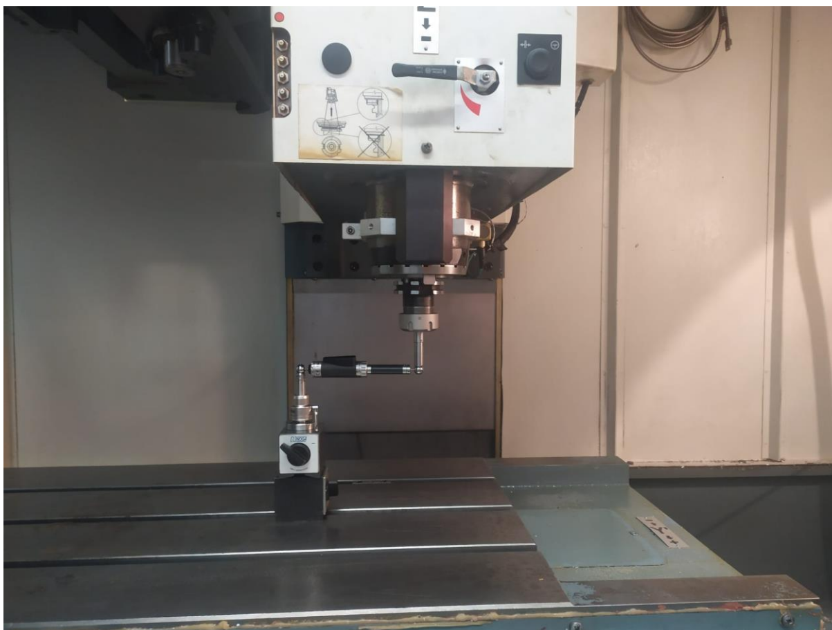
Obr. 23 Proces merania s DBB
