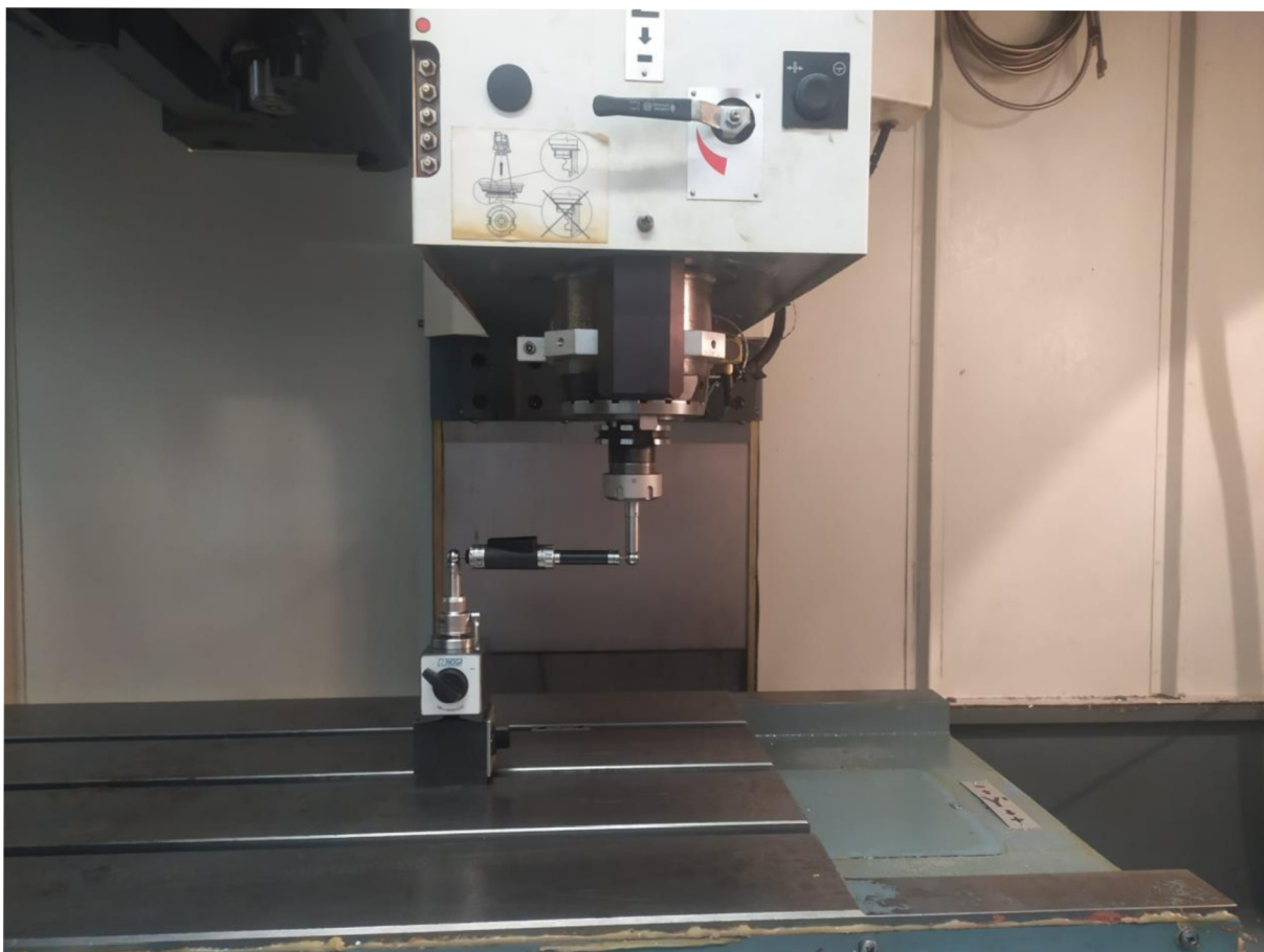
Obr. 23 Proces merania s DBB
