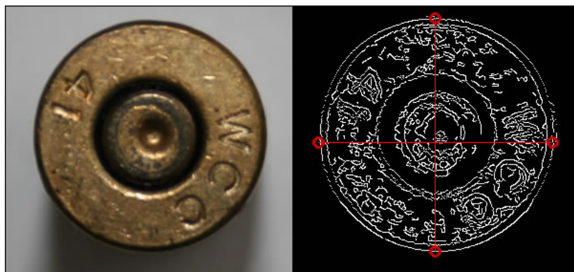
Figure 6.3: Source image of the cartridge rim and image with marked calculated dimensions.
