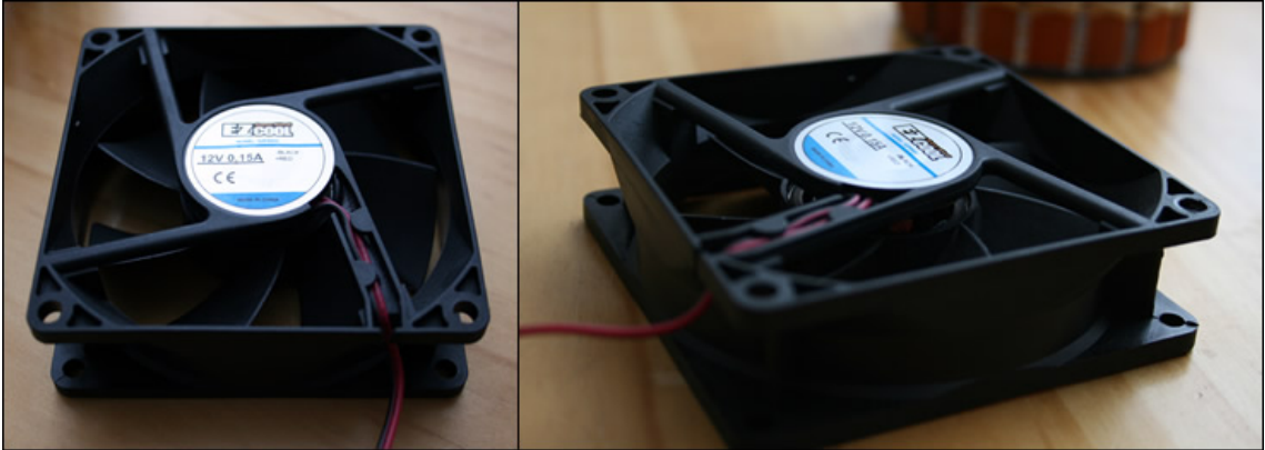
Figure B.1: EZCool EZF8025 computer cooler used as the first attempt for a rotation source in the system.
