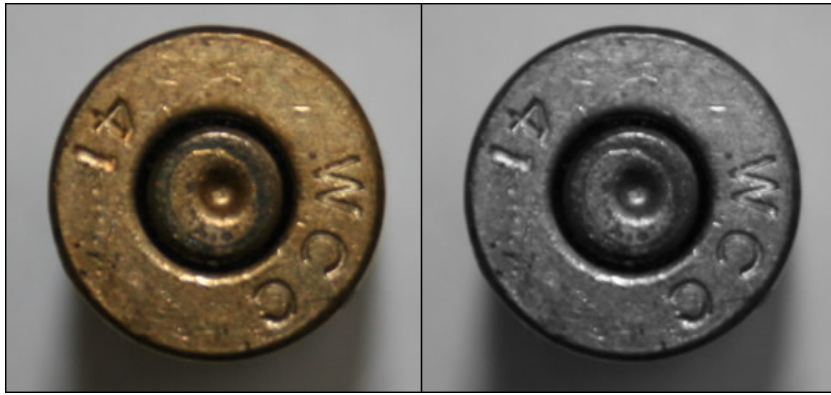
Figure 4.3: Image of a cartridge rim converted to its gray-scale version.
