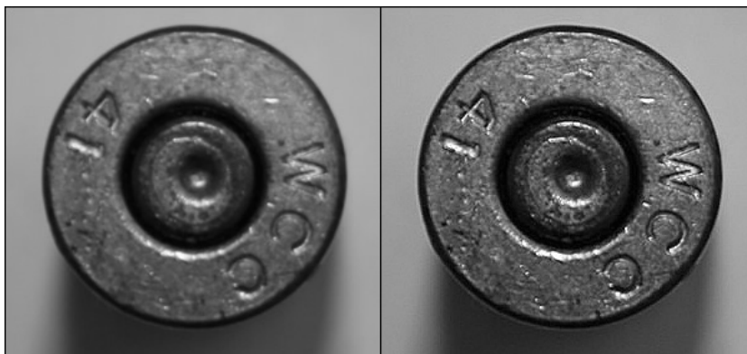
Figure 4.4: Gray-scale image of a cartridge rim and the same image after sharpening operation.
