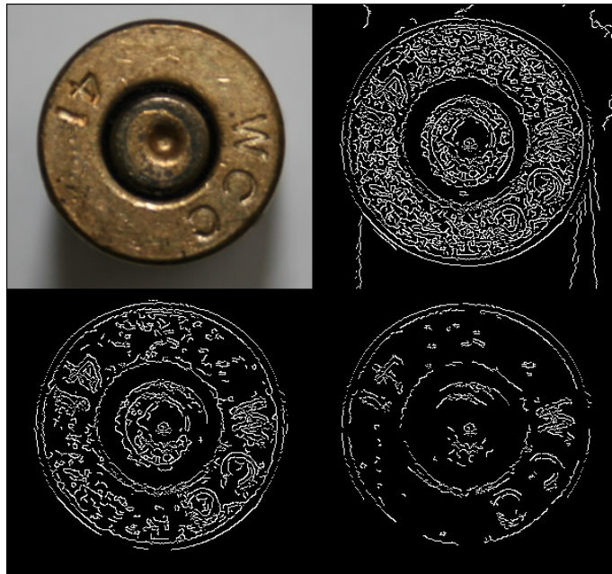
Figure 6.2: Image of a cartridge rim and the three results of application of Canny edge detector with different threshold parameters.
