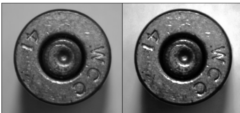
Figure 4.5: Gray-scale image of a cartridge rim before and after the histogram equalization.
