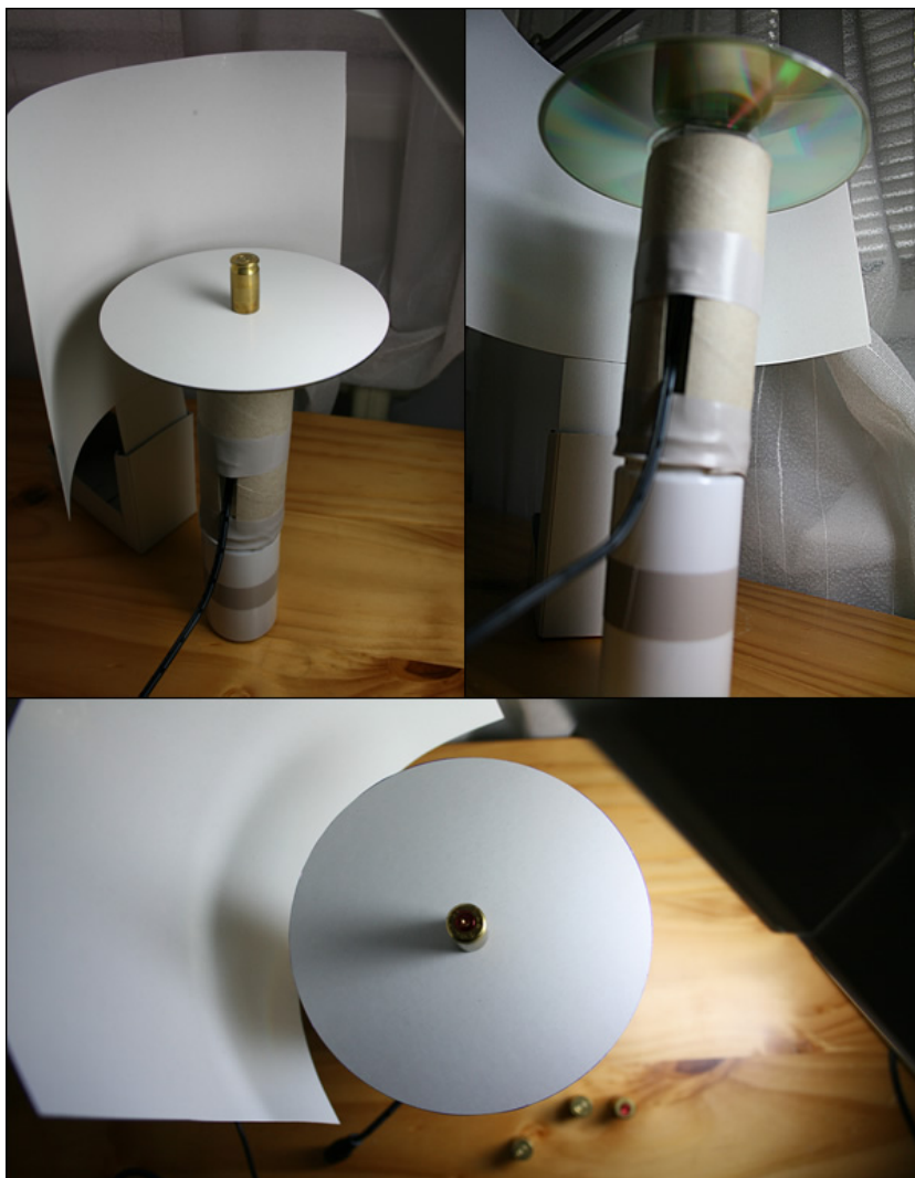
Figure B.3: Constructed mechanism with separated light source in three different views.
