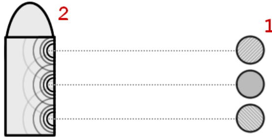
Figure 5.4: Unwanted patterns created on the surface of the cartridge case after using three directional light sources with small dispersion: 1 – Three different light sources horizontally positioned, 2 – The cartridge case with the highlighted light intensity on its surface.
