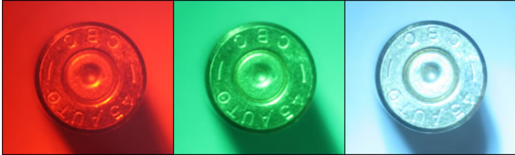
Figure 5.7: Three images of a cartridge rim, each one taken with different color filter applied in the path of light
