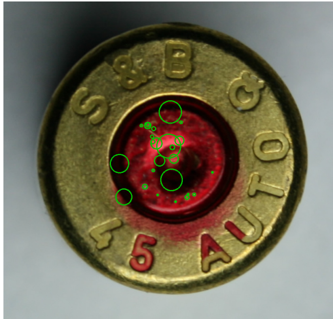
Figure 6.4: Image of a cartridge rim with extracted salient points by SURF algorithm.
