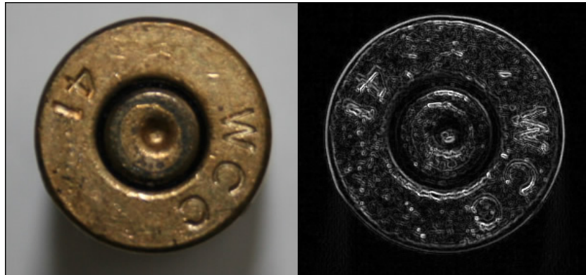
Figure 4.6: Gray-scale image of a cartridge rim and the same image with applied Sobel operator.
