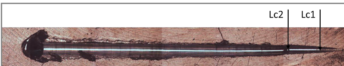
Obr. 42 Scratch test 0 – 100 N
