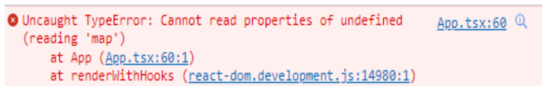
Figure 6: Run time error because of undefined data
