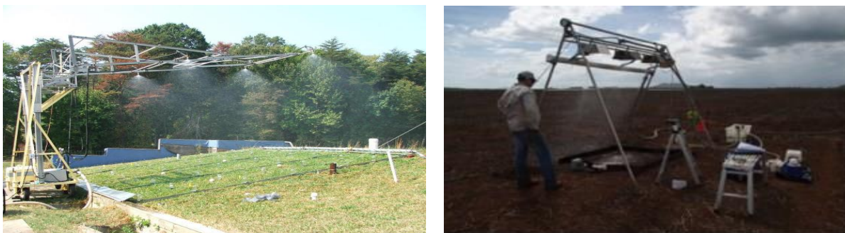
Figure 4: showing nozzle type rainfall simulator. Source: https://www.ars.usda.gov/northeast-area/beltsville-md/beltsville-agricultural-research-center/emfsl/docs/environment and http://catchmentsolutions.com.au/water-quality/
