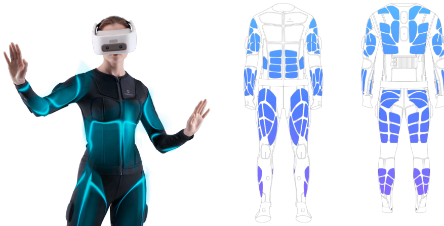
Figure 2.15: Teslasuit image (left), and a scheme of haptic stimulations (right) 28 .
