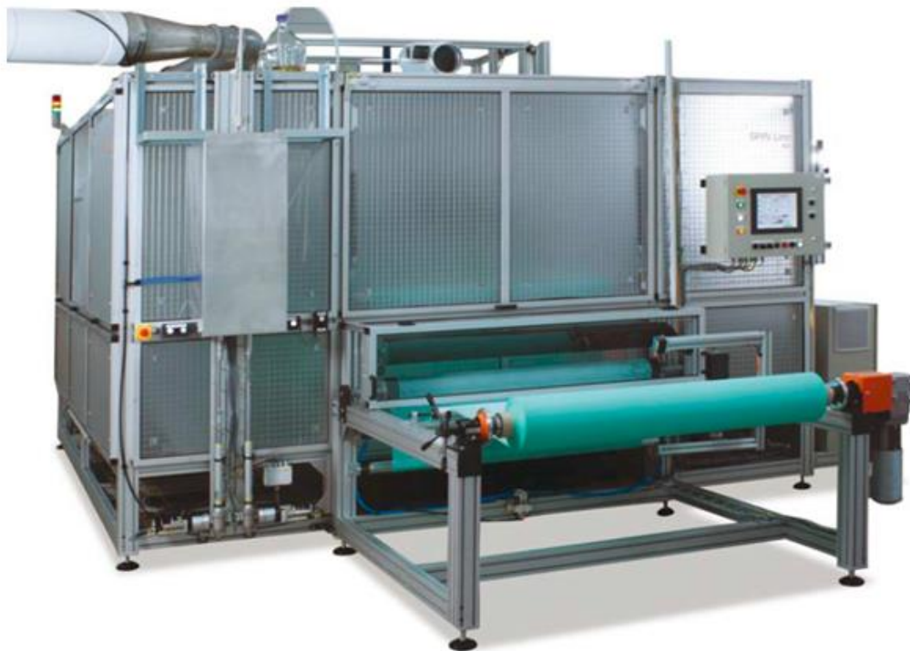
Figure 6: Unit on producing nanofiber textiles, Spin Line 120, Manufacturing width 1400 mm. (Source: SPUR a.s., Zlín)
