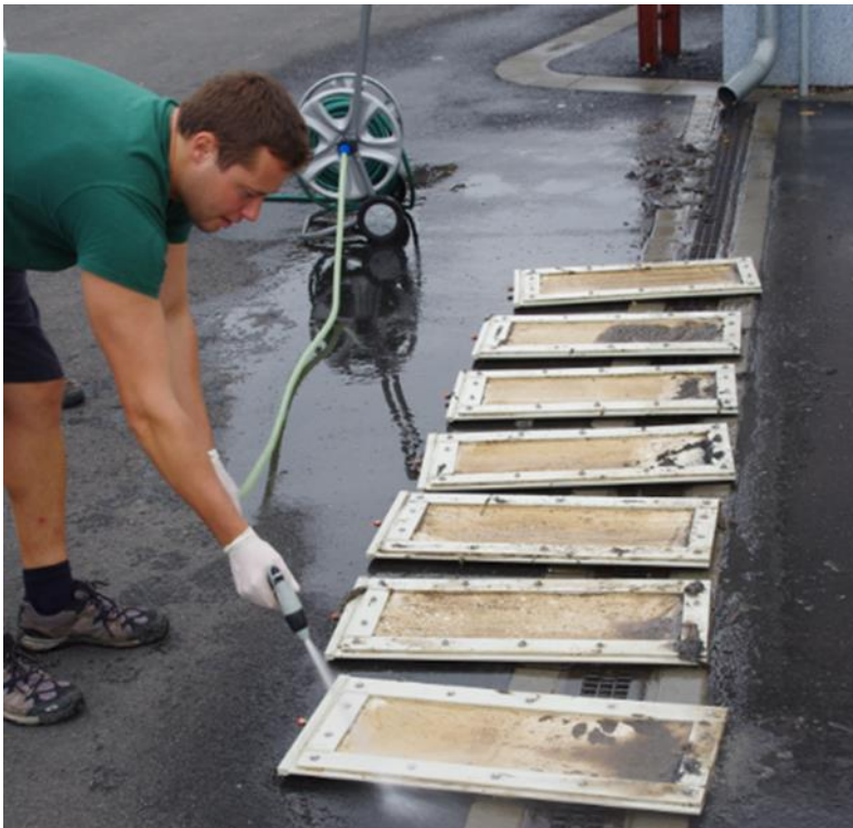
Figure 56: The first stage regeneration is spraying with clean water
