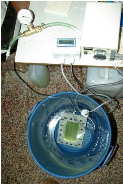
Figure 39: Testing of the flow rate of filter plate 200 x 100 mm with material labelled as: n. 94
