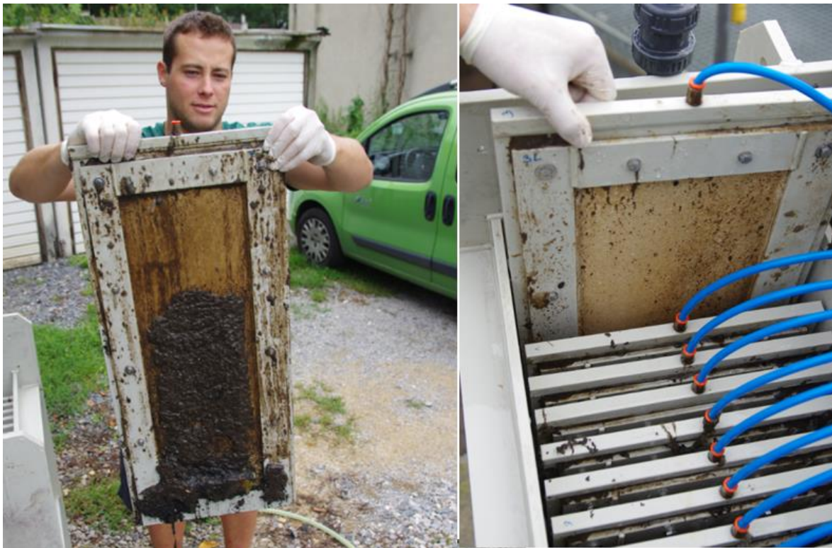
Figure 55: One of the membranes after the end of the experiment, regeneration process
