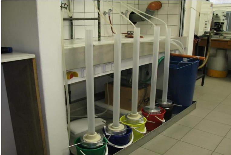
Fig. 28: Measuring the flow rate of the membranes at a constant pressure drop of 7.5 kPa
