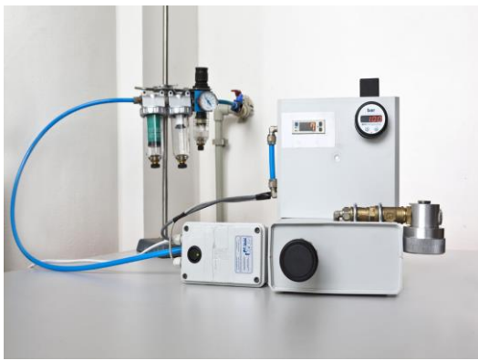
Fig 27: The assembled apparatus for measuring pore sizes and variances, SPUR a.s
