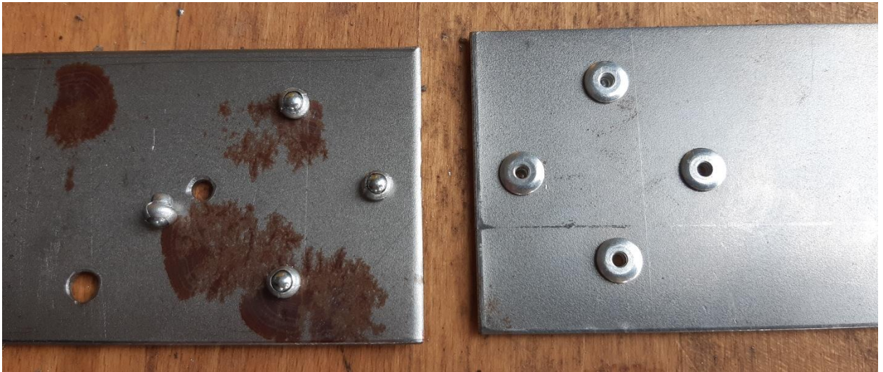
Figure 59. Eccentric configuration lap joint after static test.
