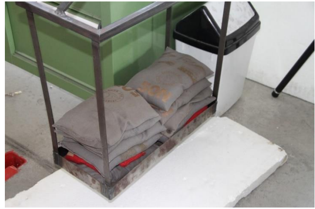
Figure 57. Static test of the eccentric configuration joint
