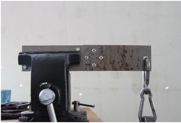
Figure 57. Static test of the eccentric configuration joint
