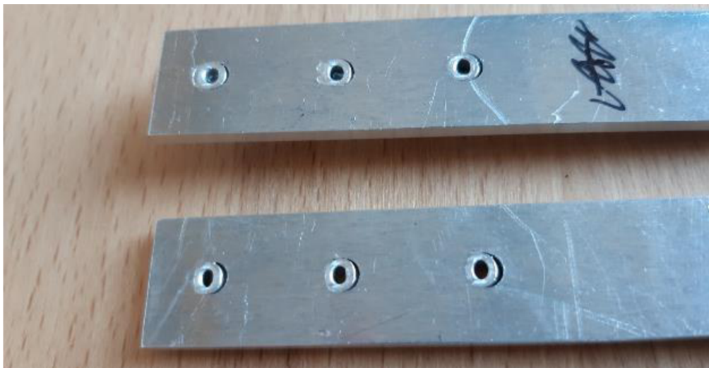
Figure 51. Three rivets in serial configuration after static test
