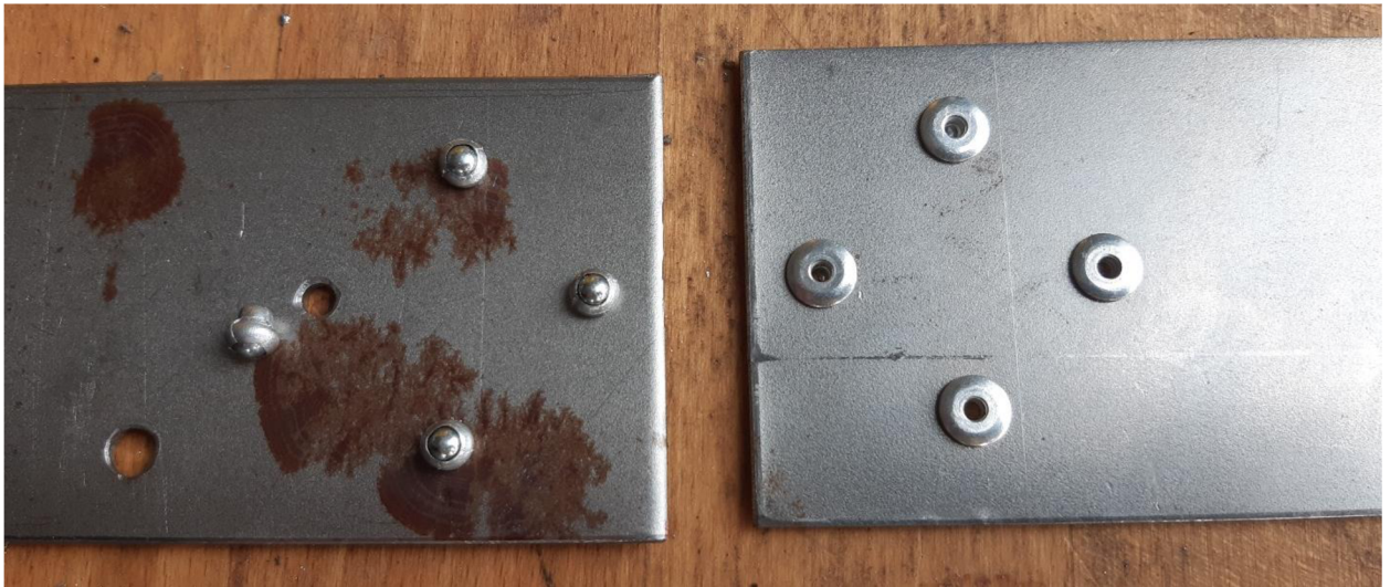
Figure 59. Eccentric configuration lap joint after static test.
