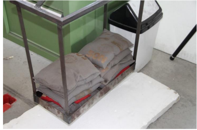
Figure 57. Static test of the eccentric configuration joint
