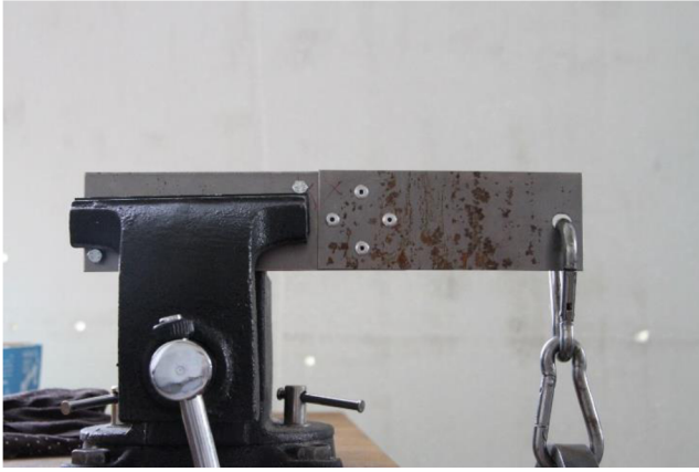
Figure 57. Static test of the eccentric configuration joint
