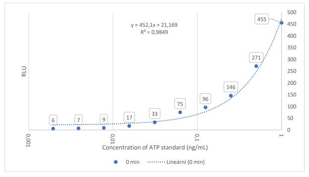
Figure 9: Standardization curve for the SystemSURE Plus kit
