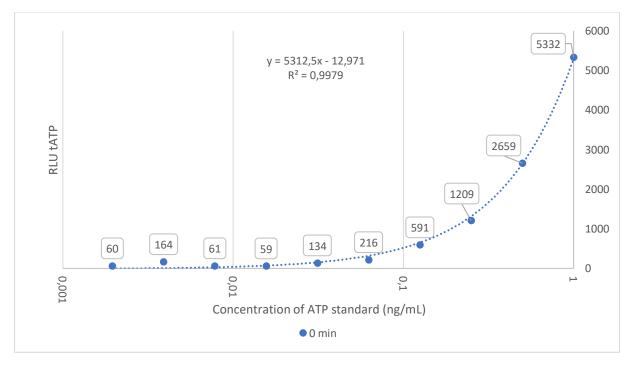
Figure 6: Standardisation curve for the DeltaTox kit
