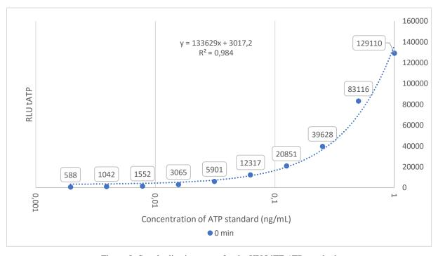
Figure 8: Standardization curve for the HY-LiTE ATP standard
