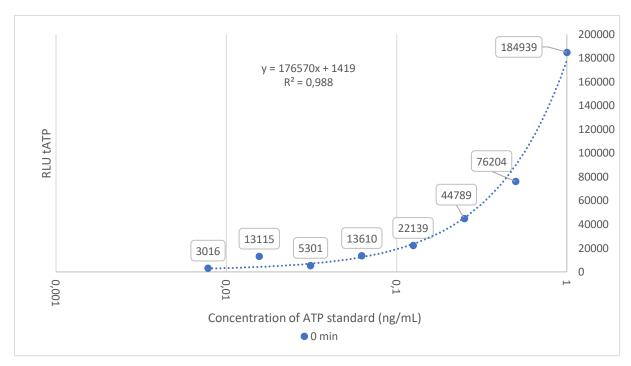
Figure 7: Standardization curve for the FLAA ATP standard
