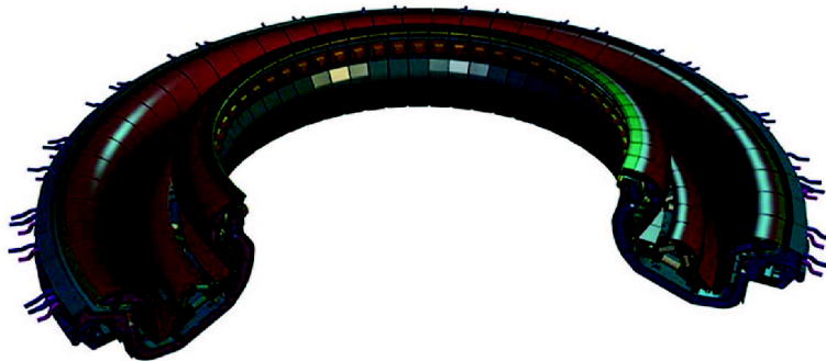
Figure 4: Cross section through the ITER divertor [1]
