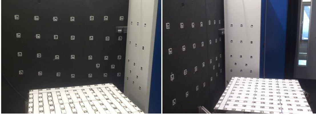
Addendum 20: Example of photographs of completely overlapping measurement. All reference markers (on the wall and locker) are visible in each image
