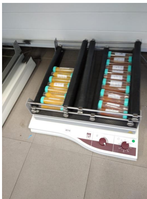
Figure 10: Laboratory shaker with Ferrihydrate samples on the right and Goethite samples on the left
