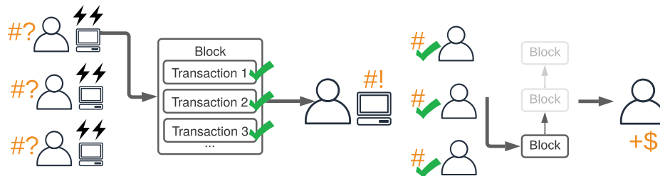
Figure 2.7: Proof-of-work consensus mechanism.
