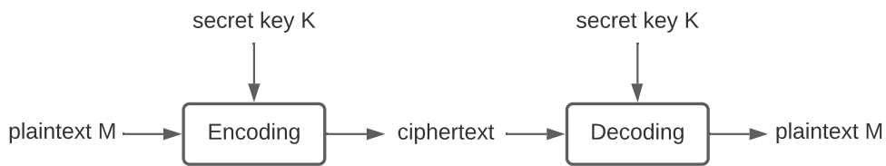
Figure 2.1: Diagram of the symmetric encryption.
