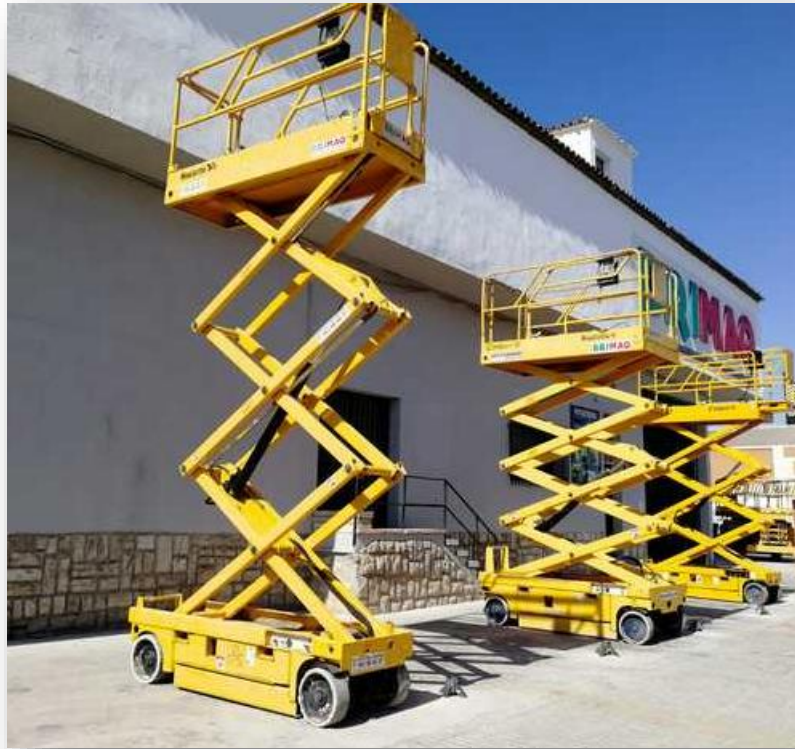
Image 2. Mobile scaffold in mechanical scissors
