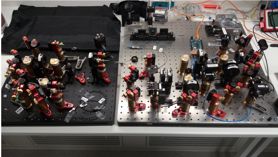
Figure A.1: A photograph of the experimental setup. Alice's setup is on the right and Bob's setup on the left. They are connected only with the short optical fiber without any added attenuation.
