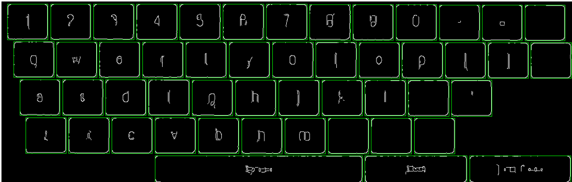
Figure 2.2: Contours and their bounding boxes can be computed from the binary image.
