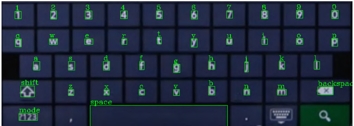
Figure 4.17: The post-processing is completed by incorporating the Canny detection results, namely the space key.
