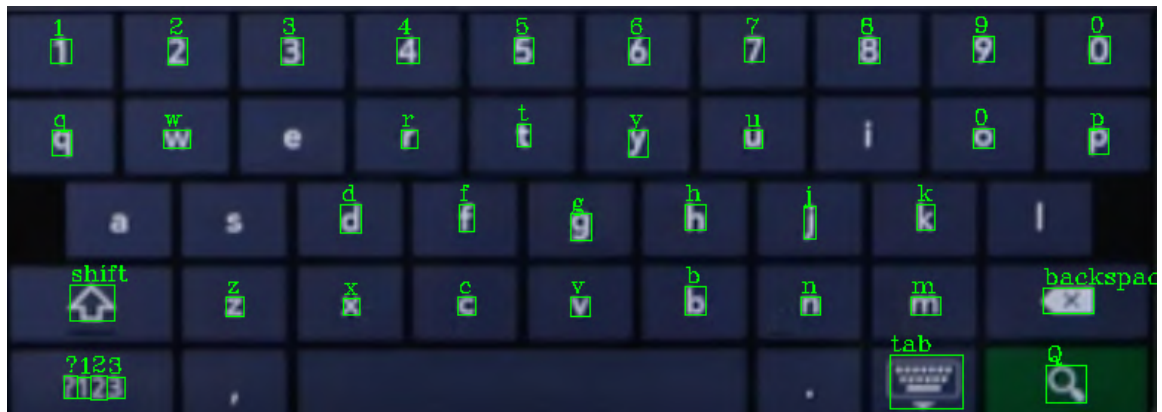
Figure 4.15: Individual characters are detected in the keyboard using the YOLOv7 model.
