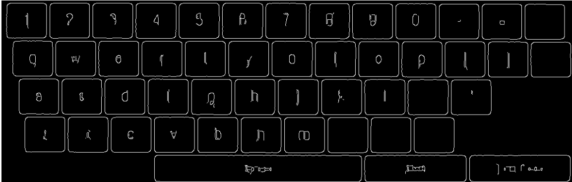
Figure 2.1: Canny detector creates a binary image with discovered edges.
