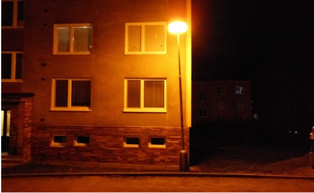
Figure 3. Example of light intrusion – wasted light spilled at the side of the residential building.
