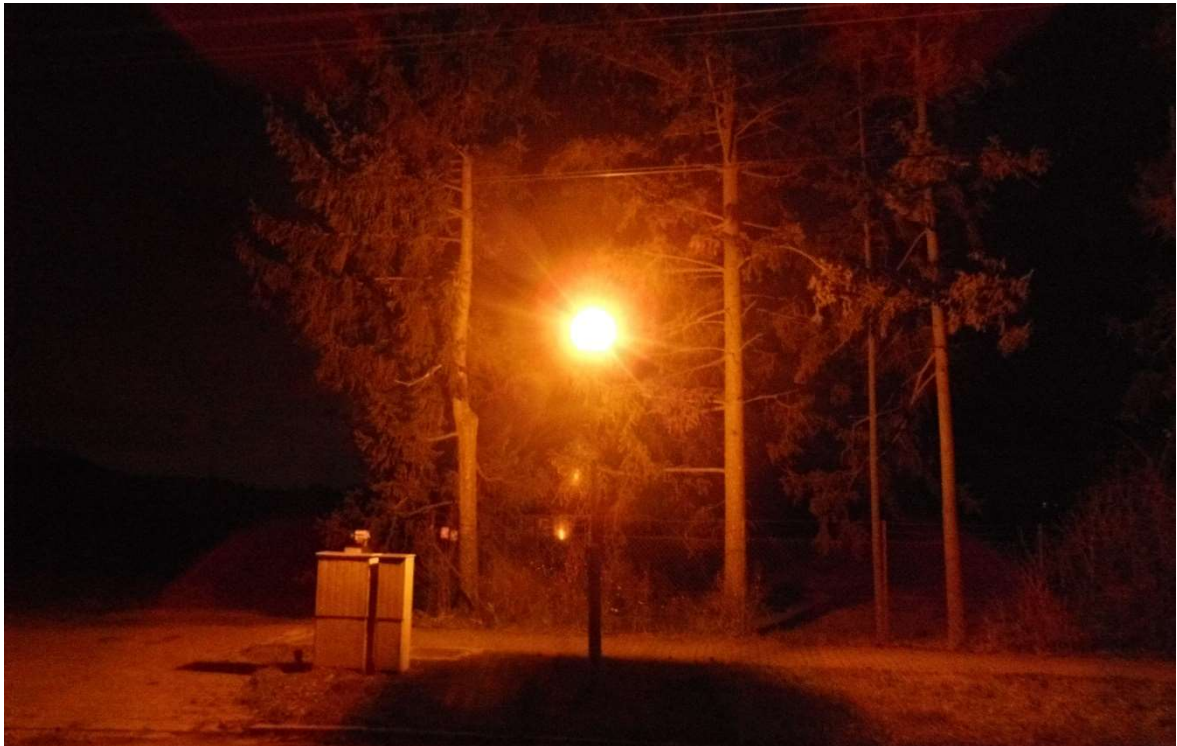
Figure 7. Wasteful design in a street light: unnecessary illuminating of the trees above.
