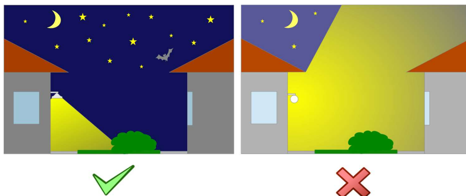
Figure 15. Example of acceptable and unacceptable outdoor luminaires. Reprinted from Odborná skupina pro tmavé nebe (2017c).
