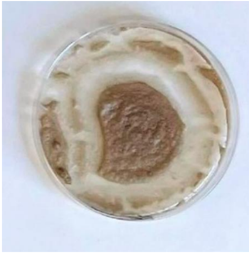
Figure 14. Biofilm from potato starch and protein (1:1), using glycerol (Tůmová 2023)
