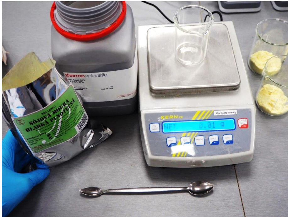
Figure 5. Weighing of raw materials for casting method (Tůmová 2023)
