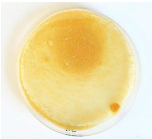
Figure 12. Biofilm from flaxseed without centrifugation (Tůmová 2023)
