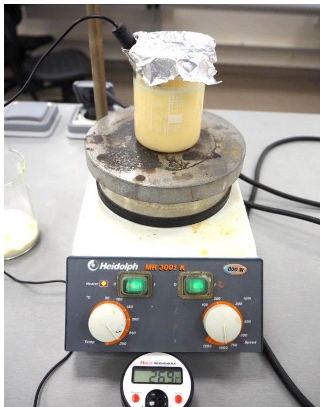
Figure 6. Heating, stirring and temperature control of the suspension (Tůmová 2023)
