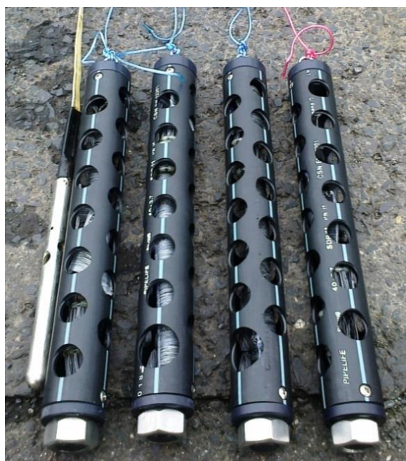
Fig. 2: Black high-density polyethylene tubes with nanofibre carriers inside.
