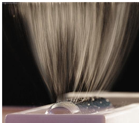
Fig. 16: Electrospinning from a free liquid surface on a rotating electrode (Petrik and Maly, 2009).
