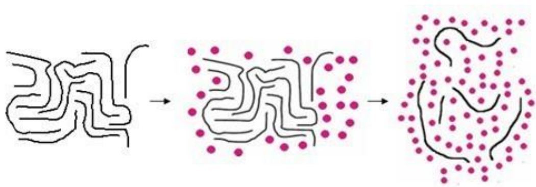
Fig.10: Model of the polymer dissolution, the diffusion of solvent molecules among the polymer chains and their solvation
