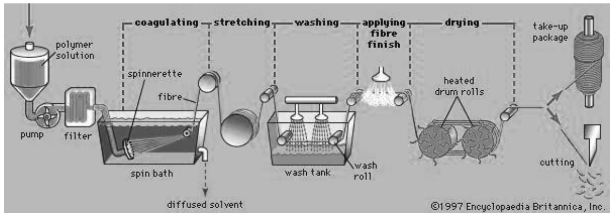
Fig.7: The wet-spinning process scheme [63]
