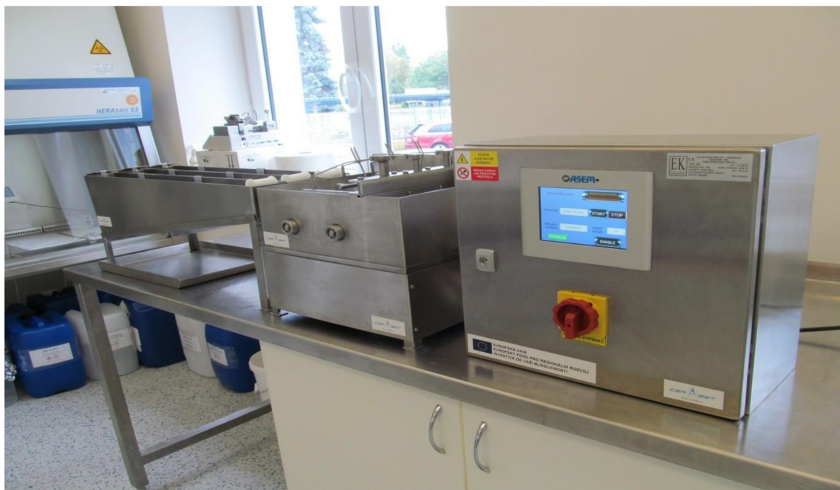
Fig 20: Laboratory wet-spinning device 3 rd generation, (Běťák, J., 2015, the final design and construction by the company CERBET [91]), Based on the agreement with the Contipro a.s., the technical details of the device are intentionally not shown.
