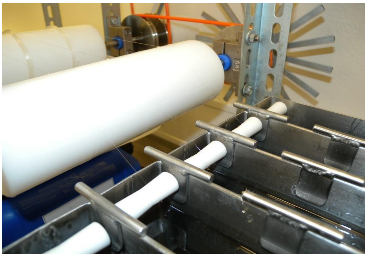
Fig 19: Laboratory wet-spinning device 2 nd generation, Extension to a triple-fiber production (Běťák, J., 2012)
