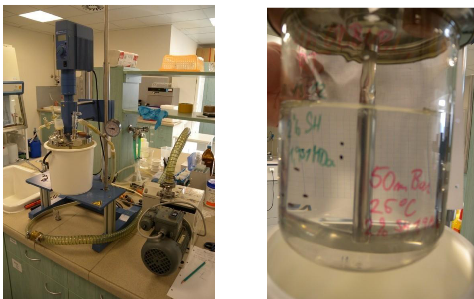
Fig.41: The trials of the vacuum deaeration process in the 2l-stirred reactor
