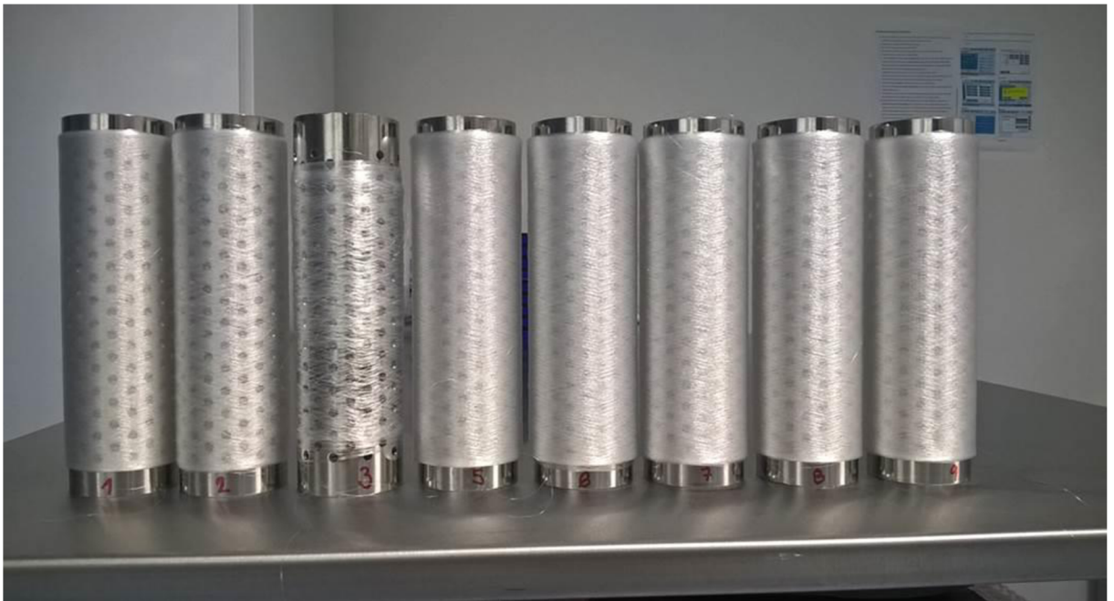
Fig.50: The first trial of the production-scale line. A paralell production of 9 HA fibers (1 fiber was lost during the rewinding).
